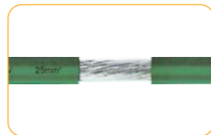
Piercing effect of wire core
